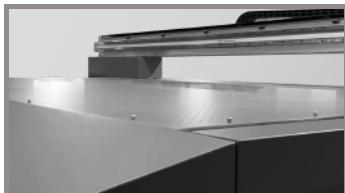
Built-in media alignment pins, guarantee the quick, simple and high precision media positioning.
