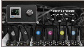
Two advanced separate negative pressure systems. Simply and effectively ensure the continuous ink flow, and easy maintenance for multi-heads equipment.
