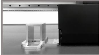
Anti-collision system is equipped to protect the printhead and carriage all the time.
